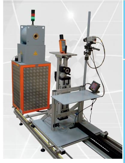
AT110 Gamma beam irradiator with calibration bench is designed for verification, calibration and examination of ionization radiation measurement instruments in collimated field of gamma radiation.
