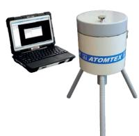
Measurement results are displayed on Information processing unit (PU) screen in real time.
