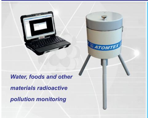
Highly sensitive selective wide-range spectrometric scintillation gamma activity monitor is intended for measuring volumetric (specific) radionuclide activity in <sup>131</sup>I, <sup>134</sup>Cs, <sup>137</sup>Cs, <sup>40</sup>K, <sup>226</sup>Ra, <sup>232</sup>Th samples with 1 litre Marinelli beaker and 0.5 litre and 1 litre flat containers.
