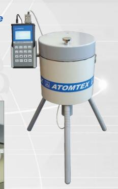
AT1320M Gamma activity monitor is a fixed scintillation radiometric unit, designed to measure volume gamma-radiation activity of <sup>51</sup>Cr, <sup>99m</sup>Tc, <sup>111</sup>In, <sup>123</sup>I, <sup>125</sup>I, <sup>131</sup>I and <sup>201</sup>TI radionuclides in liquid radioactive waste.
