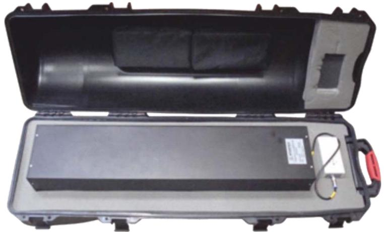
AT6103/2 Mobile Radiation Scanner in transport case
